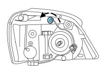
4. To remove the *parking/turn* bulb, turn the socket on the bottom of the headlamp assembly counterclockwise and pull the bulb straight out of the socket.
